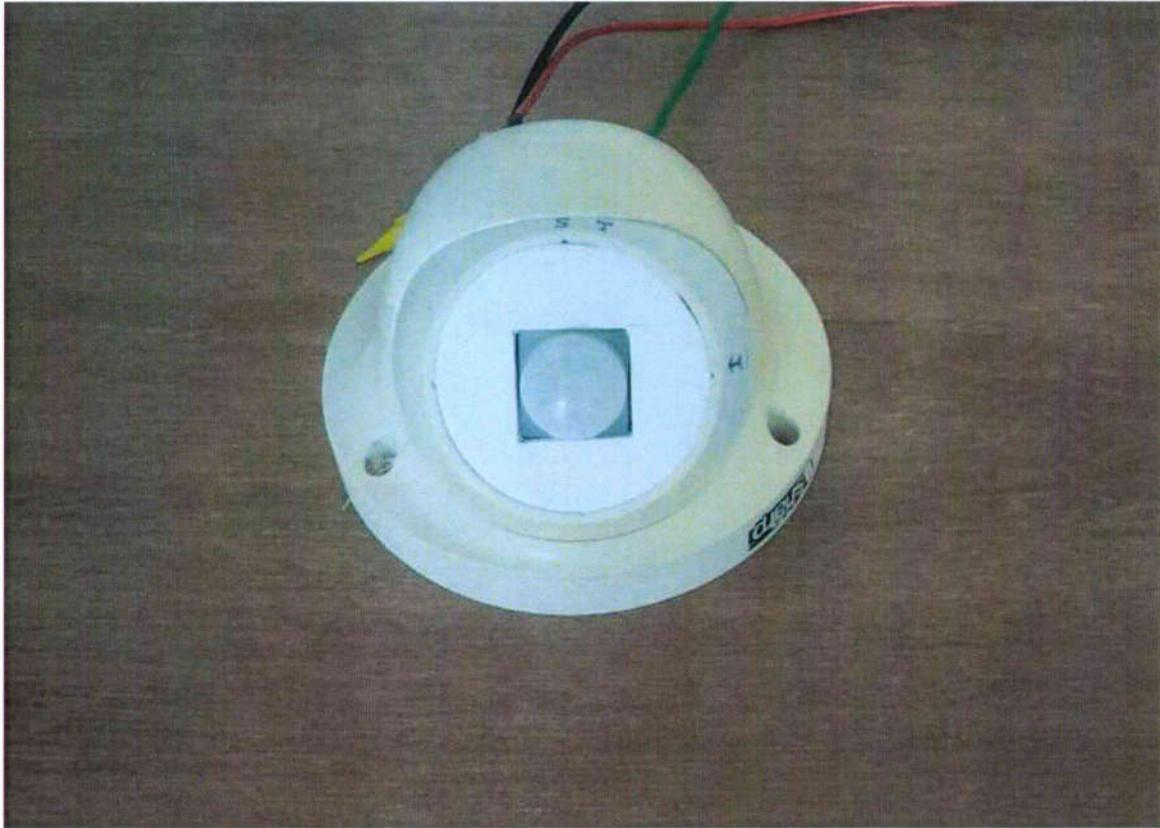
**Sensor Based Automatic Light turn On/Off Model in IOT Lab**
