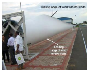
3.5 Large Wind Turbine Rotor Blade: This 600 kW blade is ready to be despatched to the wind farm for installation. The people near the blade depict the sheer size.
