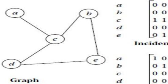
$\begin{bmatrix} 0 & 0 & 1 & 0 & 0 \\ 0 & 0 & 1 & 0 & 1 \\ 1 & 1 & 0 & 1 & 0 \\ 0 & 0 & 1 & 0 & 1 \\ 0 & 1 & 0 & 1 & 0 \end{bmatrix}$ Incidence matrix  $\begin{bmatrix} 1 & 0 & 0 & 0 & 0 \\ 0 & 1 & 0 & 0 & 0 \\ 0 & 0 & 1 & 0 & 0 \\ 0 & 0 & 0 & 1 & 0 \\ 0 & 0 & 0 & 0 & 1 \end{bmatrix}$
