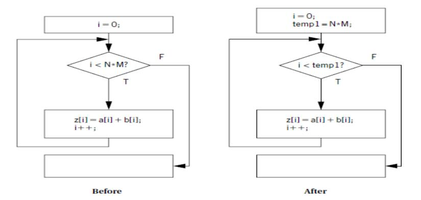
•The loop bound computation is performed on every iteration during the loop test, even though the result never changes.
