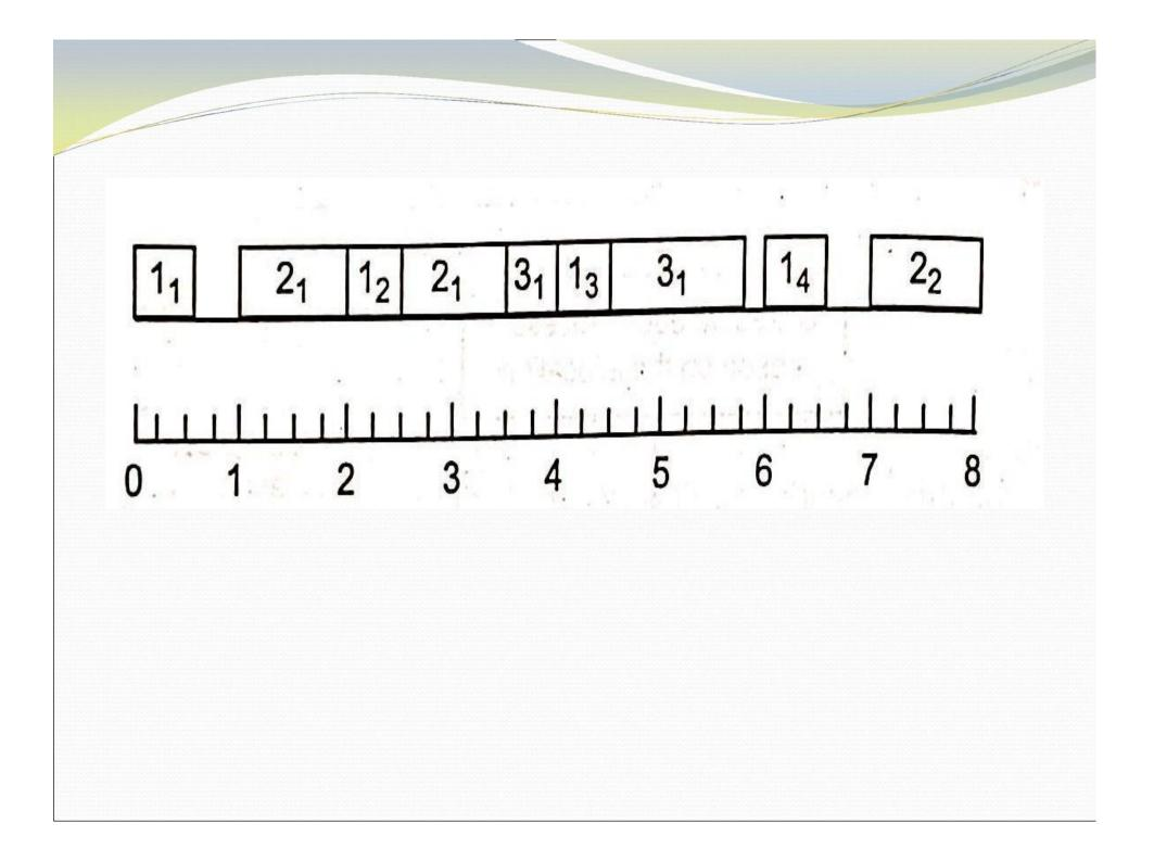
There are three tasks, with  $P_1 = 2$ ,  $P_2 = 6$ ,  $P_3 = 10$ . The execution times are  $e_1 = 0.5$ ,  $e_2 = 2.0$ ,  $e_3 = 1.75$  and  $I_1 = 0$ ,  $I_2 = 1$ ,  $I_3 = 3$ . Since  $P_1 < P_2 < P_3$ , task  $T_1$  has highest priority. Every time it is released, it preempts whatever is running on the processor. Similarly, task  $T_3$  cannot execute when either task  $T_1$  or  $T_2$  is unfinished.
