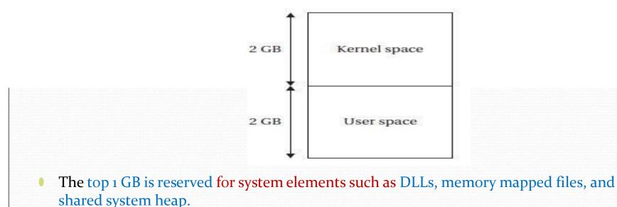
• The bottom 1 GB holds user elements such as code, data, stack, and heap.
