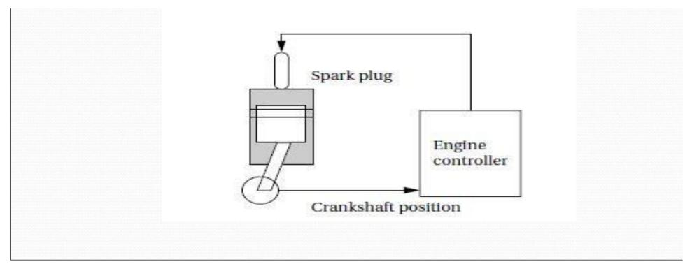
• The simplest automotive engine controllers, such as the ignition controller for a basic motorcycle engine, perform only one task—timing the firing of the spark plug, which takes the place of a mechanical distributor.
