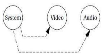
•The system decoder process demultiplexes the audio and video data and distributes it to the appropriate processes.
