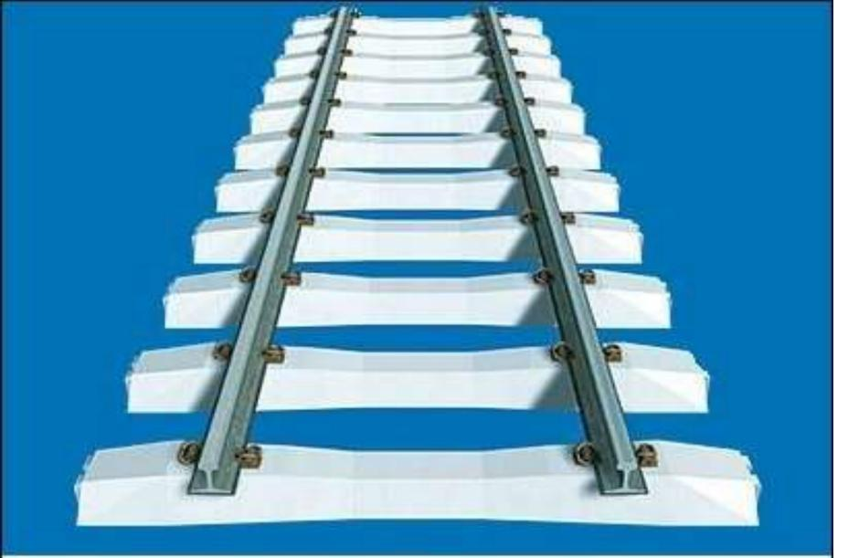
Typical arrangement of concrete sleepers with flat bottomed rail and pandrol clips. Note how the sleepers are shaped to provide a degree of natural drainage.
