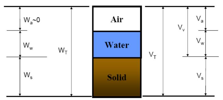
Wt: total weight Ws: weight of solid Ww: weight of water Wa: weight of air = 0 Vt: total volume Vs: volume of solid Vw: volume of water Vv: volume of the void
