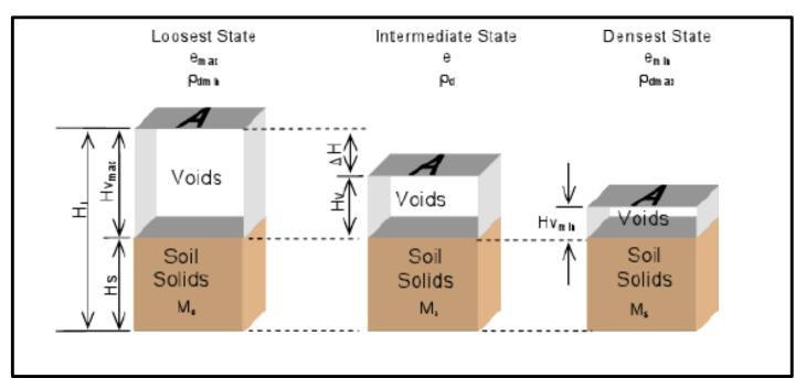
Volume reduction from compaction of granular soil
